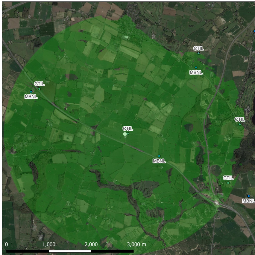
LOS modelling at 23m AGL to a target height of 1.8m above surface level
